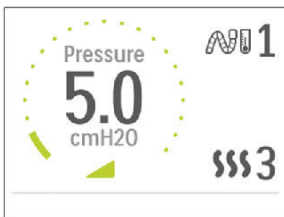
Ramp Pressure Screen
