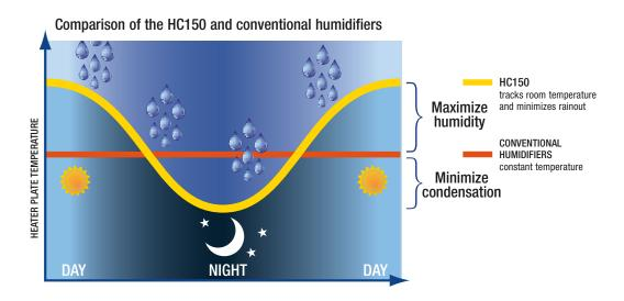
Ambient Tracking<sup>™</sup> allows the user to set the heater plate temperature higher than with a conventional humidifier without causing condensation. The user then receives more humidity during the night.
